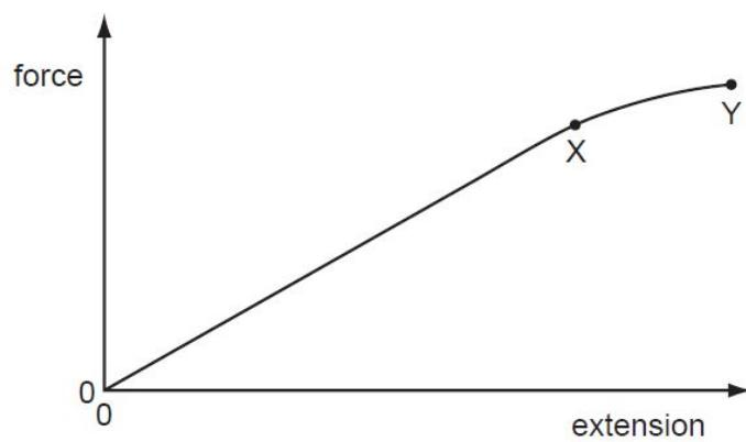
The **area under the graph is equal to the work done** in extending the material. Up until the point X, the material is extending elastically which means it obeys Hooke's law and if the force was removed it would return to its original shape and length.
