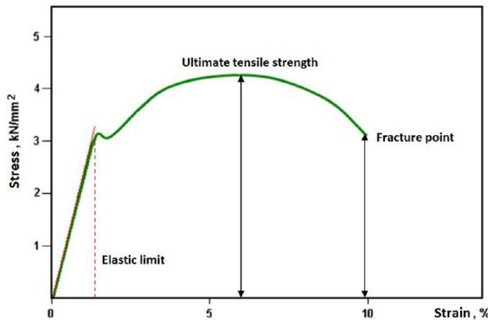
This graph shows that metals can **plastically deform for a long time** before they break (or fracture). They absorb a lot of energy before this occurs. The Young modulus is high as metals are very strong.
